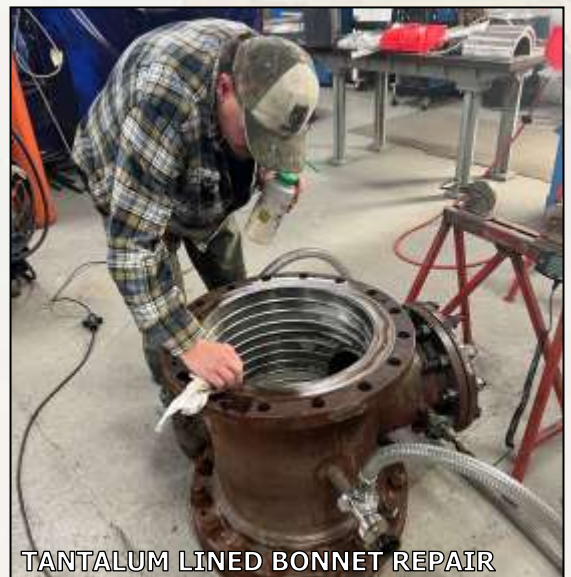
TANTALUM HEAT EXCHANGER REBUILD
