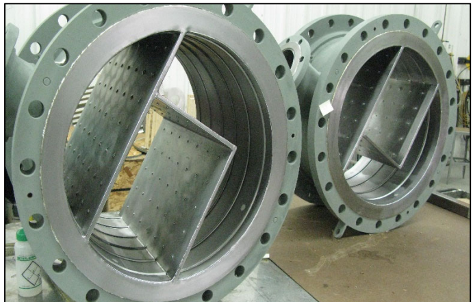
Figure 3 - Staybolts used in heat exchanger pass partition to secure tantalum lined to plate.
