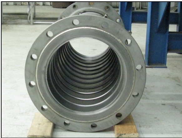
Figure 2 - Convolutions in tantalum lined pipe provide vacuum resistance and thermal expansion compensation
