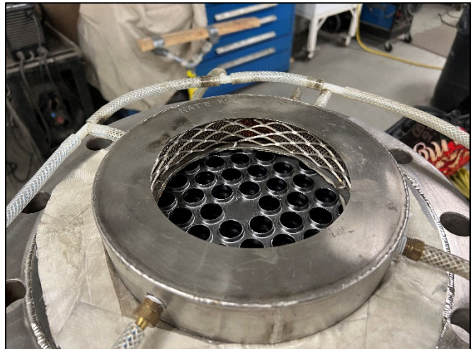
Figure 6 - Argon distributor used for tantalum welding
