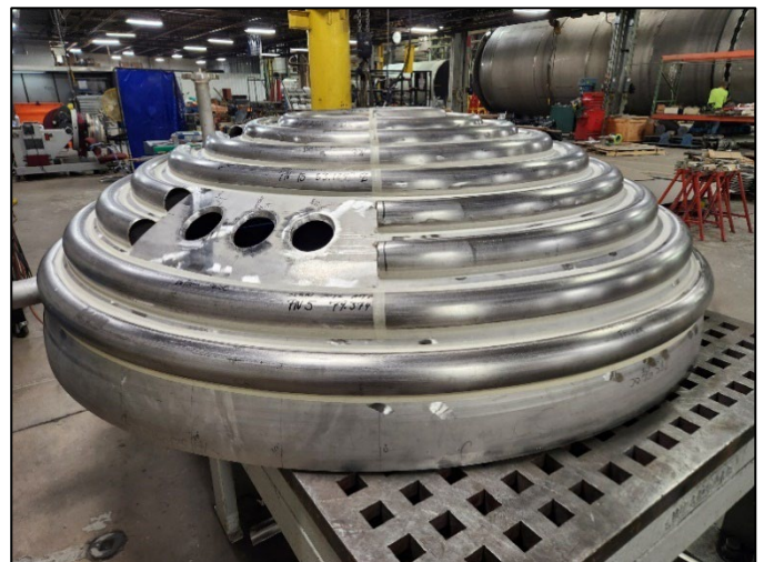
Figure 7 - Half Pipe Jacket on Pressure Vessel Head During Fabrication
