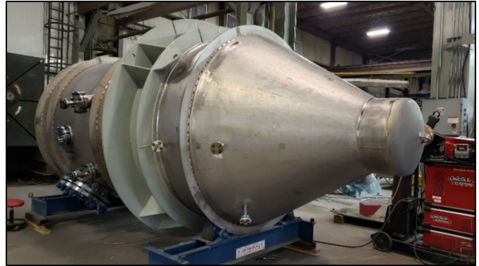
Figure 5 - Titanium Separator Vessel
