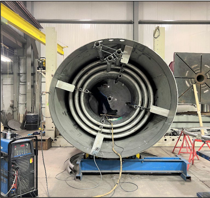
Figure 3 - Pressure Vessel with Internal Heating Coil
