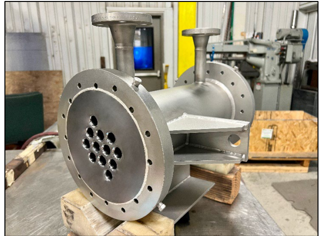
Figure 8 – Tantalum condenser with fully drainable tubesheet with 316L Stainless Steel Shell
