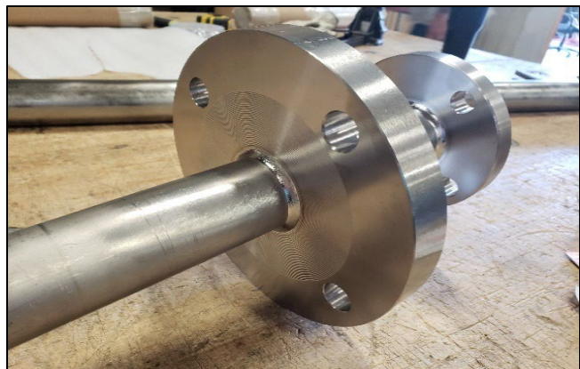
Figure 11 – Stainless Steel Dip Pipe
