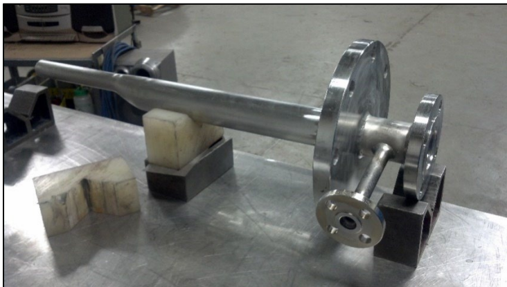
Figure 10 – Mixing Dip Pipe
