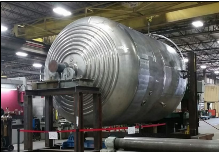
Figure 4 - Half Pipe Jacket Reactor During Fabrication
