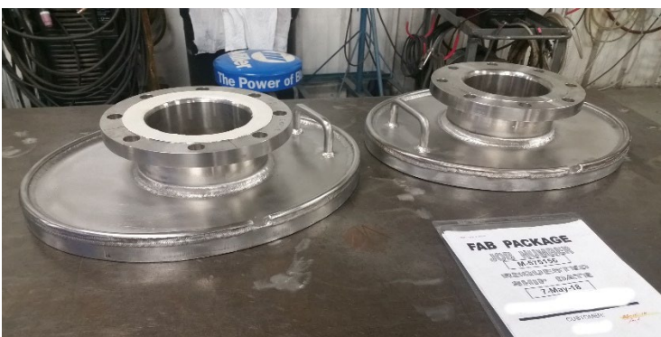
Figure 12 –316L Stainless Steel Manway Covers
