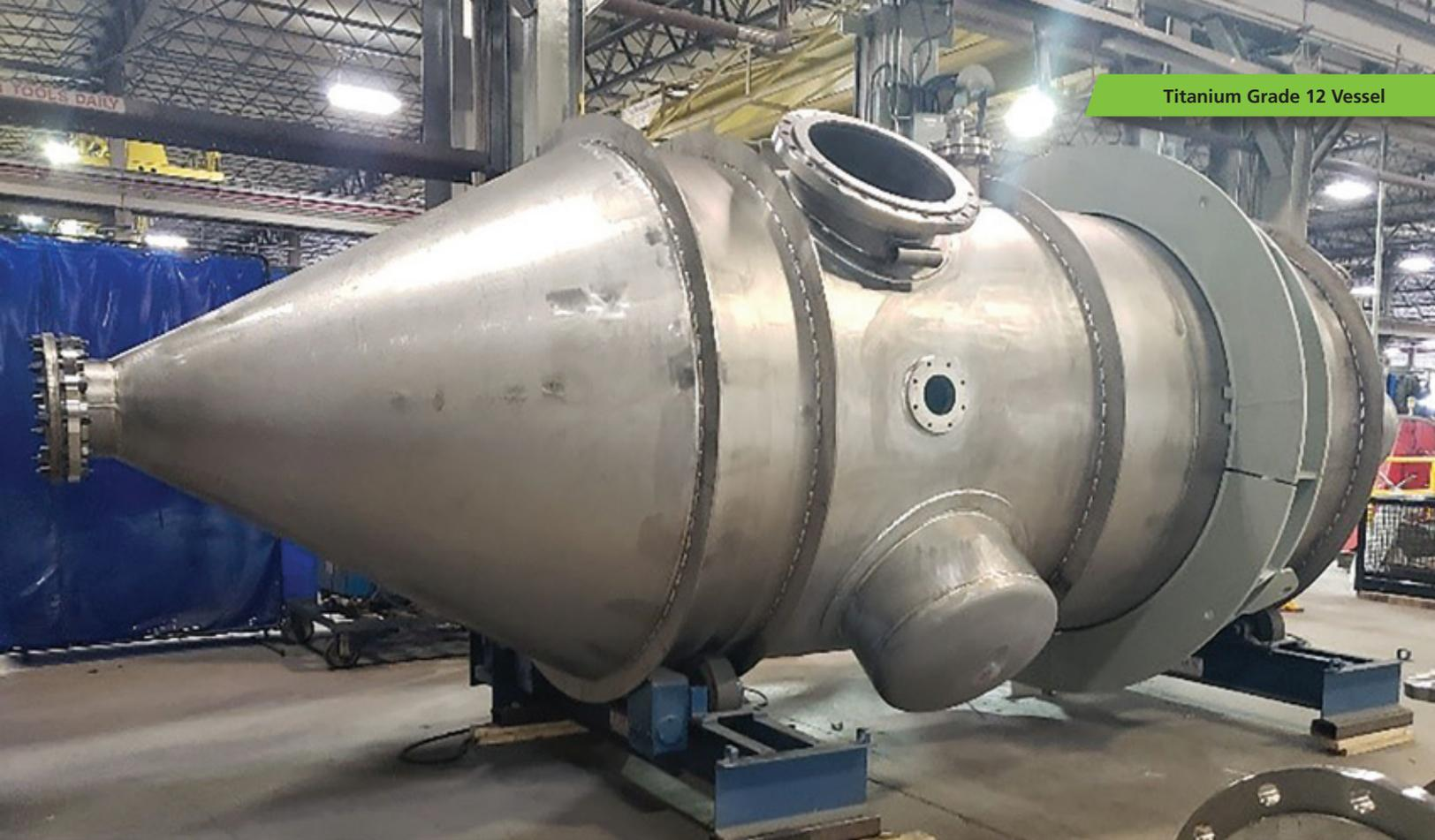
quantity justifies a special mill run), this would require a plate thickness of 0.625 inches – 5/8 in. nominal thickness. With Ti Grade 12, the thickness required would be 0.41 inches and the actual plate thickness used would be 0.4375 inches – 7/16 in. nominal thickness. Using Ti Grade 12 as an alternative to Ti Grade 2/2H would result in a savings of 30 percent of material.
