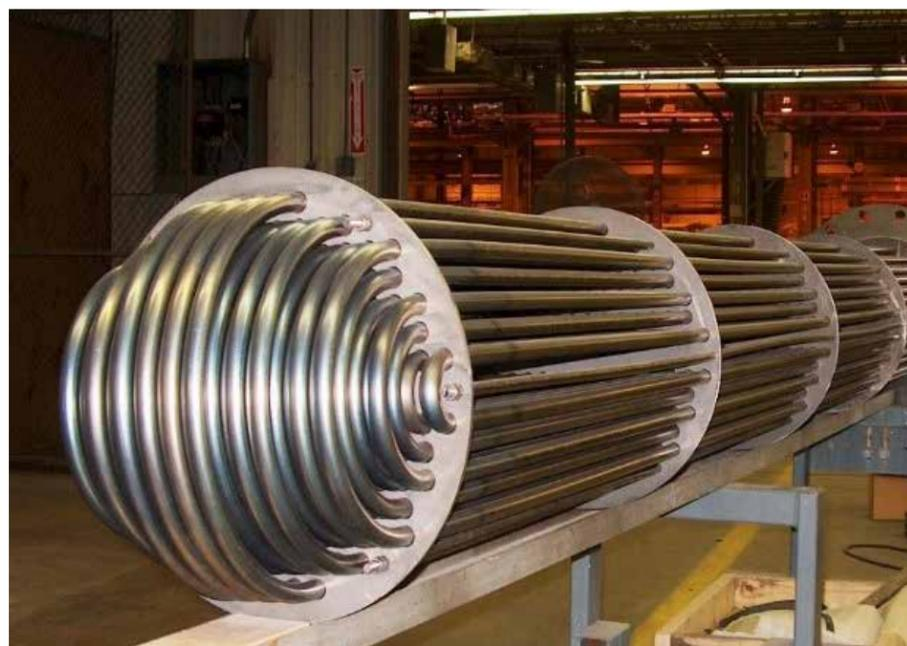
A titanium u-tube bundle. Image courtesy of Tricor Metals
