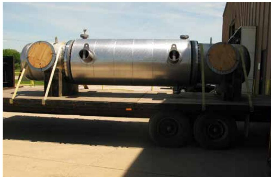
A titanium shell and tube cooler/condenser. Image courtesy of Tricor Metals
