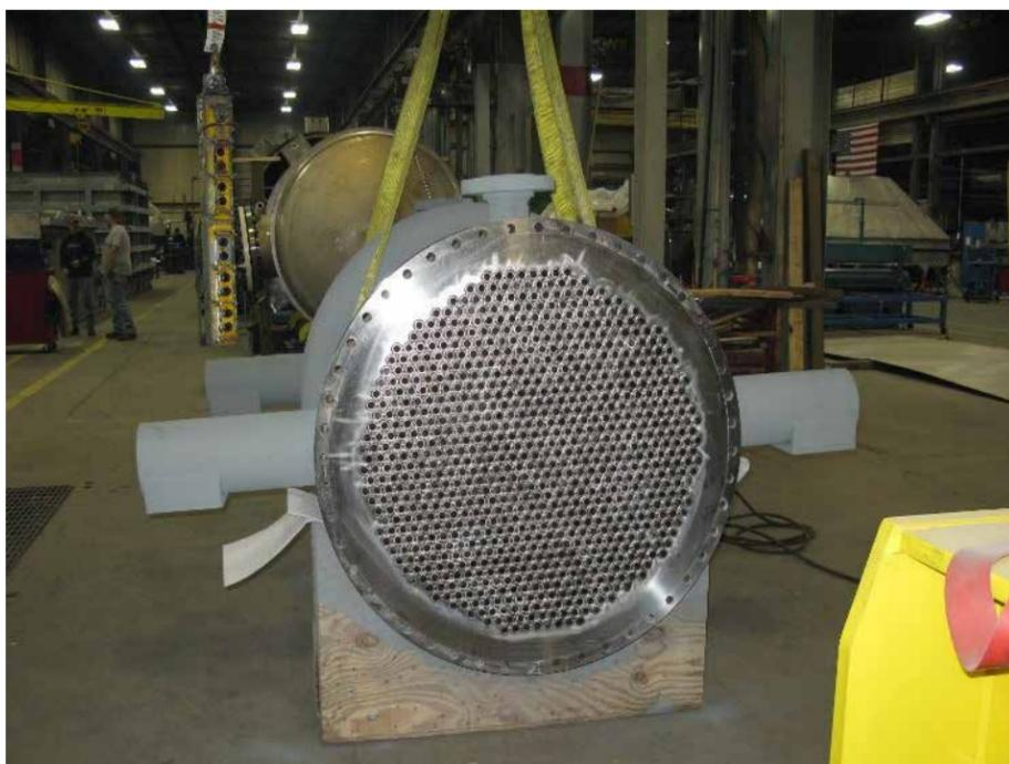
A titanium shell and tube bundle. Image courtesy of Tricor Metals
